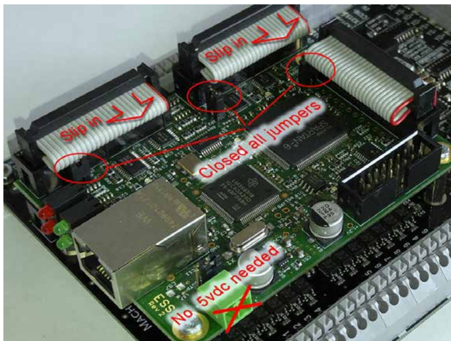
Figure 3, Jumpers are closed, No external 5Vdc
