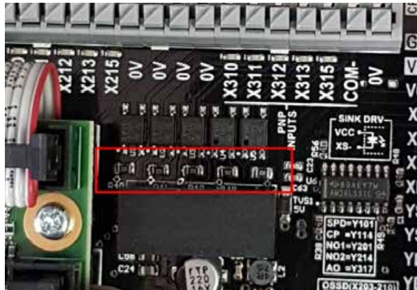
Figure 20, Replace 3k with 470 ohm resistor for PNP inputs.
