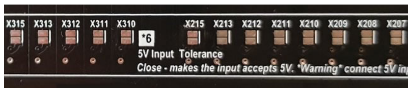
Figure 38, 5V input tolerance solder bridges.
