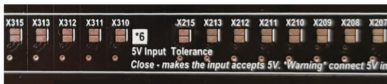
Figure 38, 5V input tolerance solder bridges.
