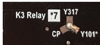
Figure 39, K3 Pin select solder bridge.
